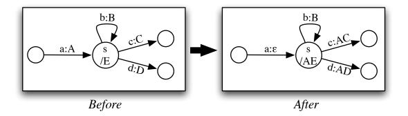
Figure 4.6: Output Delay.
